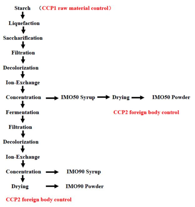
(Metal detect: iron <1.0mm; non FE <1.2mm; stainless<1.5mm)
